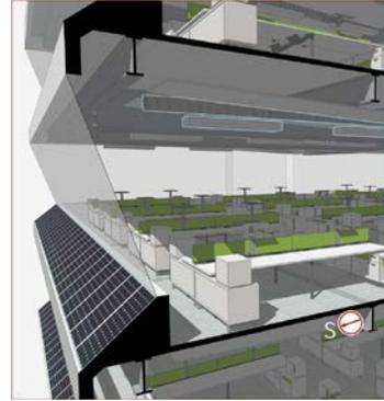
One of the simplest ways to design sustainably is to commit to utilizing sustainable construction materials wherever possible. Utilizing locally-sourced, recycled-content construction materials is an excellent means to help achieve this. An example of this consideration was a structural design team's attempt to maximize steel framing throughout the project, since steel, which contains a high percentage of recycled content, can be locally sourced from Boston steel mills.
