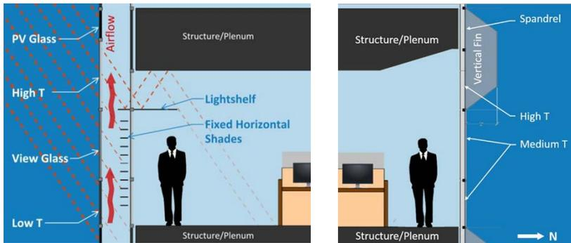
one team worked early on to maximize the floor-to-ceiling height adjacent to the façade to create a light well that will maximize daylighting. The building will be oriented approximately 20 degrees west of north, so to reduce the effects of direct sunlight striking the north façade during
