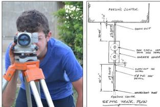
**Environmental Engineering:** A sanitary engineer from our local Public Works assisted us in determining the best solution for a septic tank system. Multiple alternatives were reviewed and analyzed. The final recommendation was to use two 500 gallon HDPE tanks.
