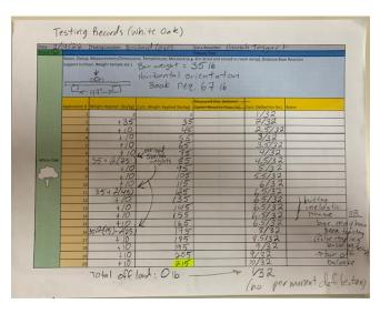
showing cumulative applied load versus resulting deflection are shown to the left. The nearly linear results also indicate minimal to no damage done to material fibers during loading, essentially elastic behavior. We loaded and unloaded our samples, taking measurements of deflection for each increment, and found that no permanent deflection existed for either species after full unloading.
