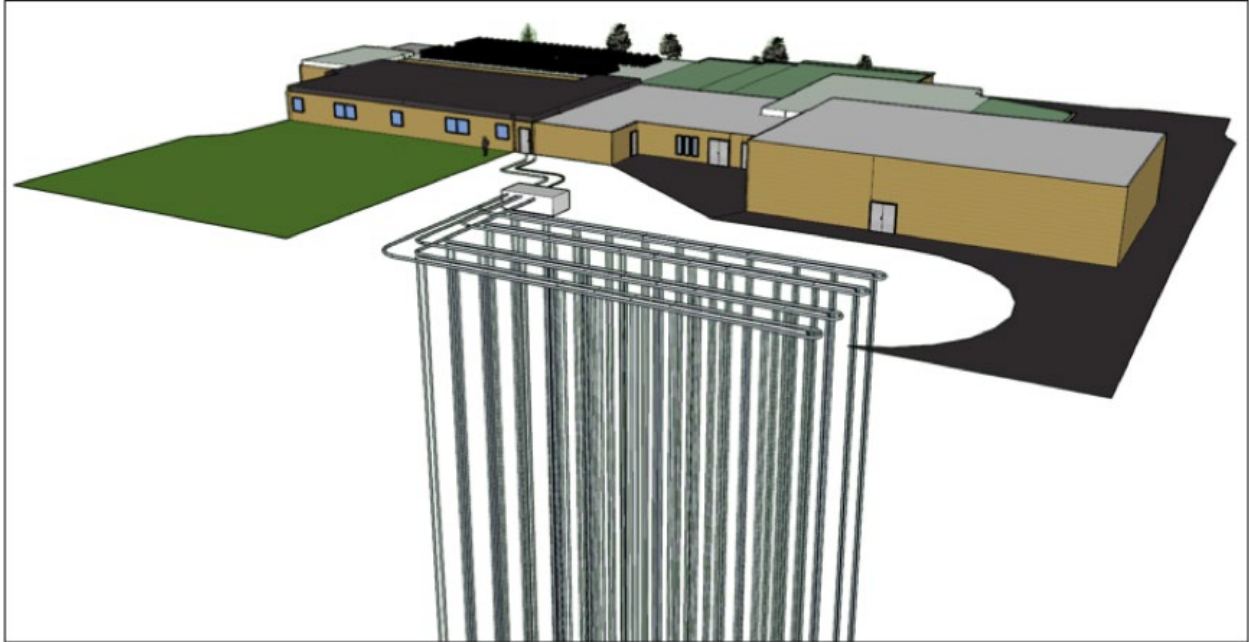
Figure 8. Rendering of the final design for the renewable energy system at School A, facing northeast (including solar and geothermal system components).
