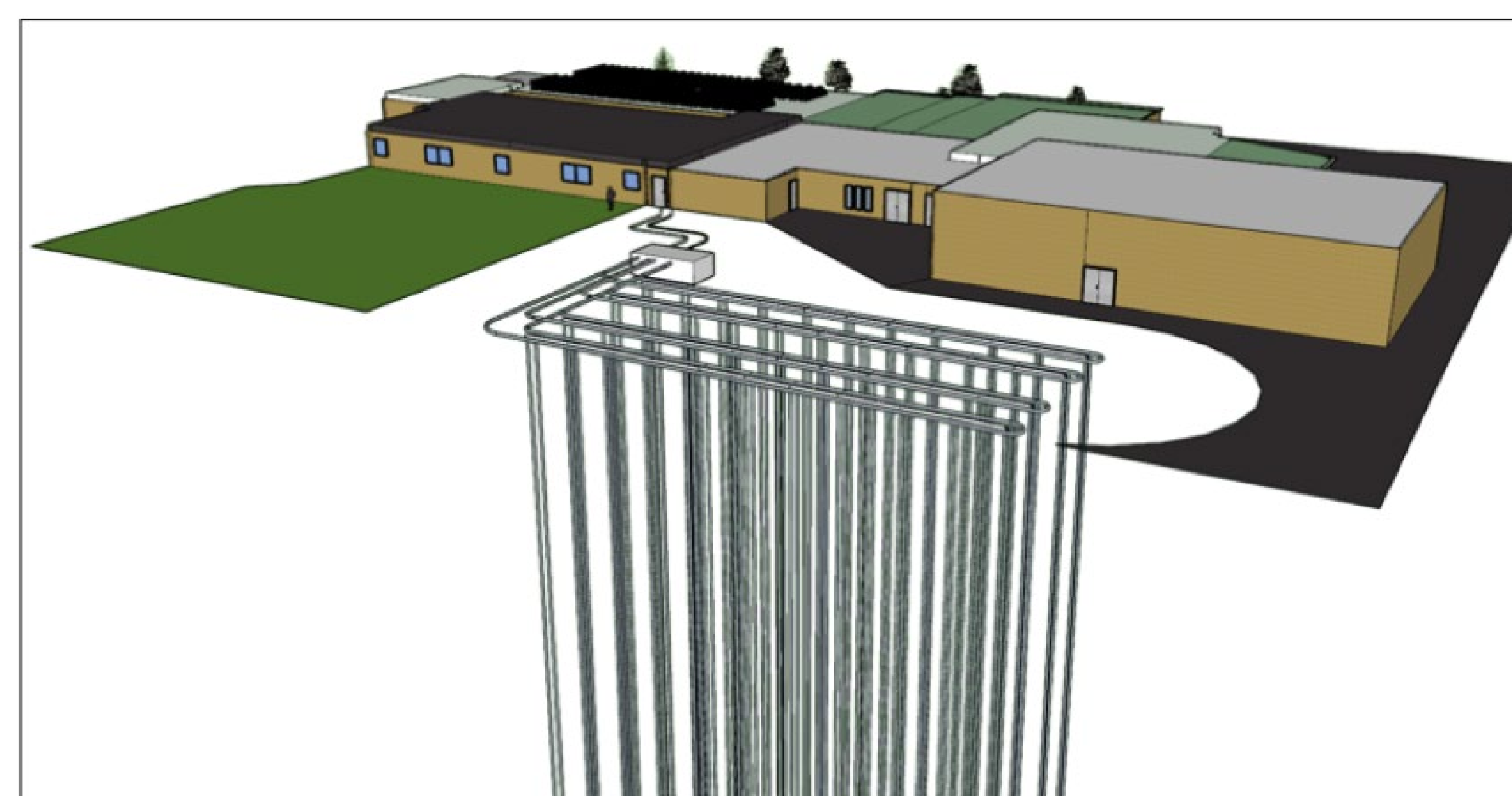
Rendering of renewable energy system at School A, facing northeast (including solar and geothermal system components)
