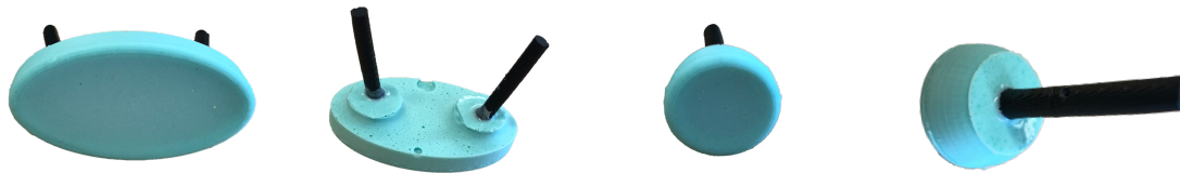
Figure 2: Final prototype of our two pads using the two types of silicone
