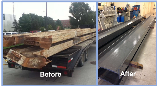
Figure 5: Photos of the steel beams before and after cleanup
