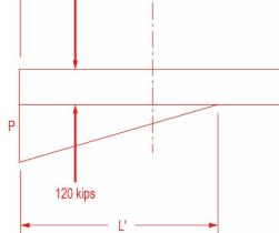
Resultant of soil pressure must align with eccentric resultant load. L' is the effective length of the triangular soil pressure pattern.
