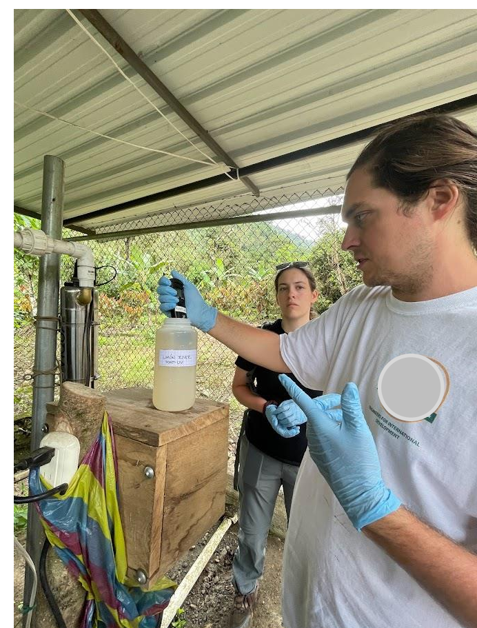
A student testing the turbidity in the water supply after the UV system
