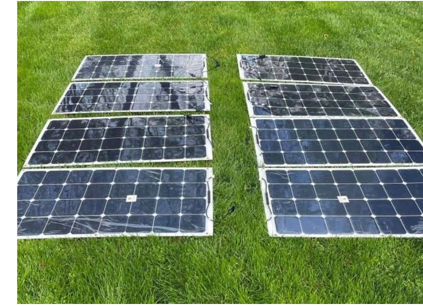
Field testing of the (800W at 48-Volts) Solar Array in the USA
