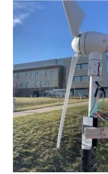
Field testing the wind turbine in the USA (150W at 12-volt) system
