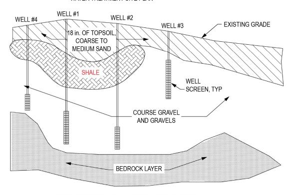
HYDROGEOLOGIC CROSS-SECTION OF WELL FIELD
