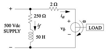
For a particular field strength, the back emf  $v_b$  is directly proportional to the motor speed  $\omega$ . In steady state, under a particular load, the current  $i_a$  is measured to be 12A when the speed is 850 rpm and  $i_f$  is 2A. With field current at 2 A, if the motor were started with no additional resistance in series with the armature, the initial current  $i_a$  (amperes) would be most nearly:
