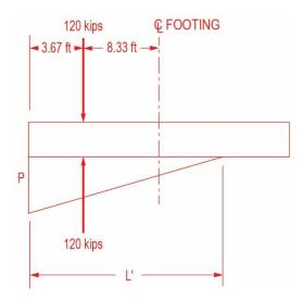
Resultant of soil pressure must align with eccentric resultant load. L' is the effective length of the triangular soil pressure pattern.
